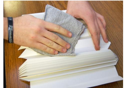
**STEP 15:** Using Viper Anti-Venom Spray-n-Wipe gently clean and wipe down each fold in the bellows.
