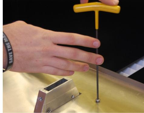
**STEP 5:** Using a 9/16" hex head, remove the four screws holding the Shirt Support Tray to the drive base. There are two in the front and two at the rear of the Shirt Support Tray.
