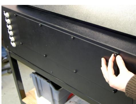
**STEP 8:** Remove the 8 thumb screws that hold the Rear Access Panel in place. This will give inside access to the rear of the Viper.
