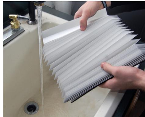
**STEP 14:** Using warm water, gently rinse off the bellows. Do not scrub. Take care not to rip or tear bellows. Replace with new bellows if damaged.
