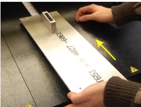
**STEP 7:** Slide the Shirt Tray Support plate to the rear to free it from the Drive Assembly. Lift to remove from the Drive Assembly.
