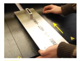
**STEP 7:** Side the Shirt Tray Support plate to the rear to free it from the Drive Assembly. Lift to remove from the Drive Assembly.
