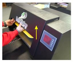
**STEP 1:** Disconnect the power cord from the Viper XPT. Remove the garage door by lifting up with both hands.
