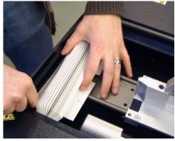
**STEP 11:** Gently release the front bellows from the velcro attachment points on the front of the Viper.
