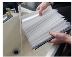
**STEP 14:** Using warm water, gently rinse off the bellows. Do not scrub. Take care not to rip or tear bellows. Replace with new bellows if damaged.
