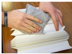
**STEP 15:** Using Viper Anti-Venom Sprayn-Wipe gently clean and wipe down each fold in the bellows.
