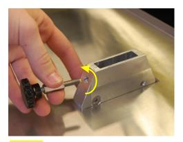
**STEP 4:** If it has not been removed completely, remove the platen support set screw.
