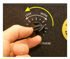
**STEP 3:** Based on the chart and the fluid lay down amount rotate the knob counter clockwise the correct number of rotations. If for example you want 30 grams of fluid, rotate the knob 1 full turn.
