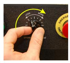
STEP 2: Start by rotating the control knob clockwise until you start to feel resistance. DO NOT OVER TIGHTEN. This is called zeroing out. If you do not know what the ViperONE Spray Control Knob is set to, zero it out and re-adjust.
