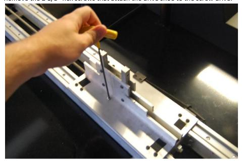
4. With the shoe released from the screw, gently slide shoe off of the front of the rails.
