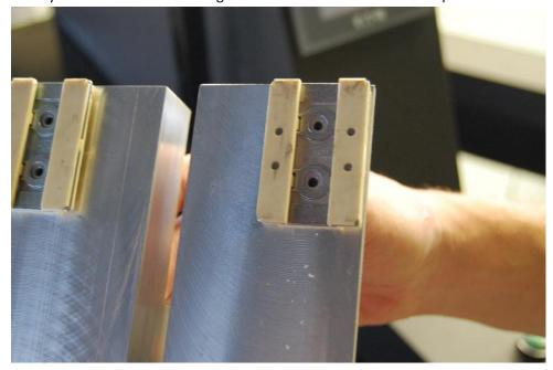
6. Teflon bearings can be removed for cleaning if needed (carefully lift up and off –see picture below). IMPORTANT: If removed, be sure to replace each bearing in the exact position it was removed from. Bearings with holes should all be on the same side.
