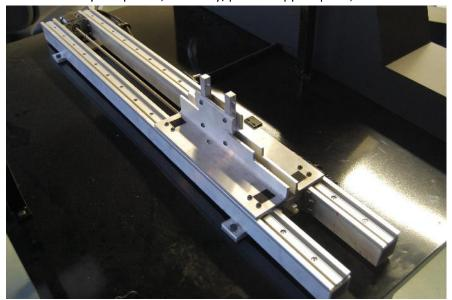
3. Remove the 2 1/8" hex screws that attach the drive shoe to the screw drive.
