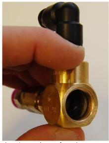
**Step 3:** Ensure there is no polymers from the pretreatment stuck in the body (#1 part below) or tube fittings of the pressure relief valve.
