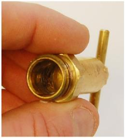
**Step 4:** Also clean and remove any pretreatment from the pressure setting side of the relief valve (#4 part below).
