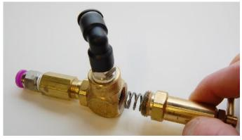
**Step 2:** Disassemble the pressure relief valve. Note the spring. The piston is located in the body of the valve directly underneath the 90 degree elbow tube fitting. See #2 in the exploded view below.
