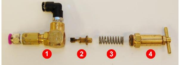
**Step 5:** The picture above shows the pressure relief valve disassembled from left to right. Ensure that you DO NOT loosen the smaller nut on #4. This holds the preset pressure setting for the valve. Adjusting this will adjust the spray pressure and spray pattern. Thoroughly clean all parts #1 through #4. When reassembling, do not over tighten #4 when retightening to the main body valve #1.
