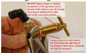
**Step 1:** Use a crescent wrench to loosen the large nut on the right side of the pressure relief valve as seen above.
