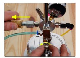
**STEP 1:** Disconnect the air source from the pressure container. Open the Air Release Valve on the pressure container to remove any pressure inside the container.
