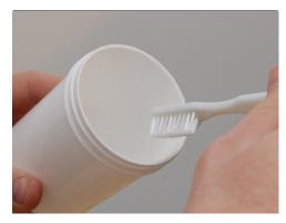
**STEP 4:** Dip the tooth brush in clean, warm water and brush the tip of the spray nozzle cleaning it thoroughly.
