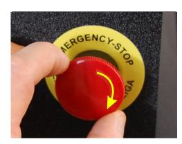
**STEP 9:** Reconnect the air source. Release the Emergency Stop Button by twisting it 1/8 turn clockwise.
