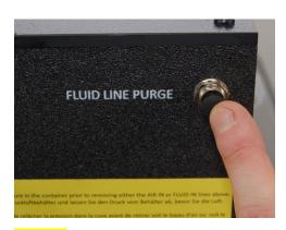
**STEP 7:** PURGE the ViperONE a couple of times to remove any residue from the spray nozzle.
