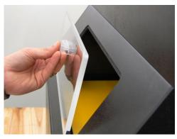
**STEP 8:** Gently move the spray carriage to the front of the ViperONE. Replace the window. Reconnect the air source.
