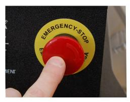
**STEP 3:** Depress the Emergency Stop button to release any air pressure in the system. Gently grab the spray tip and pull the spray carriage to the middle of the machine.
