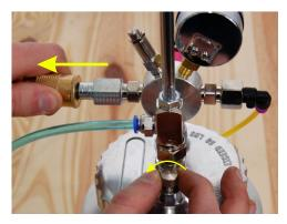
**STEP 6:** Remove the air compressor connection from the Pressure Container. Next, release the pressure in the container by opening the Air Relief Valve.
