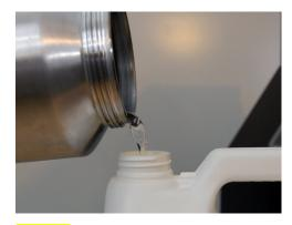
**STEP 7:** Empty the Pressure Container. Thoroughly rinse the container with water to remove any residue of Anti-Venom Maintenance Cleaning Solution.
