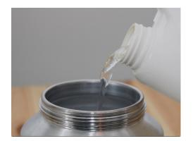
**STEP 1:** Make sure the Pressure Container is not pressurized. Empty the water from the Cleaning Pressure Container and fill container with at least .5 liter of Anti-Venom Maintenance Solution.
