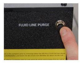
**STEP 5:** Press the PURGE button and hold for 5 seconds. Repeat 3-5 times. When done, remove the Purge Container and dispose of waste accordingly. **DO NOT ALLOW THE ANTI-VENOM MAINTENANCE SOLUTION TO SPRAY INTO THE GUTTERS INSIDE THE VIPERONE.**
