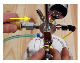
**STEP 3:** Reconnect the air compressor to the Pressure Container.
