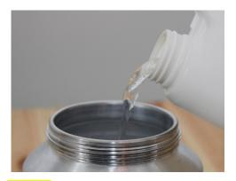
**STEP 8:** Fill the Pressure Container with distilled water and Repeat Steps 1-6. The distilled water will flush the Anti-Venom Maintenance Solution from the fluid lines.
