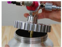
**STEP 2:** Tighten the lid back on the Pressure Container. Close the Air Relief Valve and connect the Fluid Line and Air Lines from the ViperONE to the Pressure Container.
