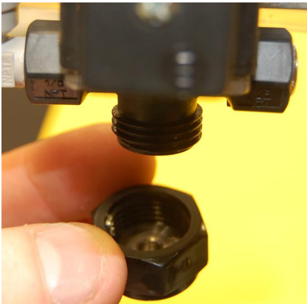
Figure 5.3.3 – Replace the tip and black nut that holds the tip
