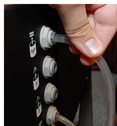
Fig. 2.3 B – Firmly insert tube.
