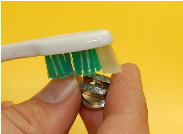
Figure 5.3.2 – Scrub the spray tips with Image Armor CLEANING SOLUTION, then rinse with warm soapy water and a tooth brush.
