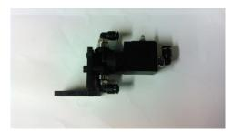
Step 1: Remove the Solenoid from the machine. Make sure to disconnect the flags and fluid lines. Note where the fluid lines go to each elbow.
