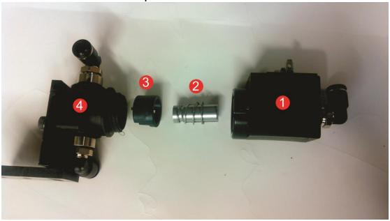
**Step 8:** The picture above shows the Fluid solenoid disassembled from left to right. Make sure to thoroughly clean every part seen above. Ensure that no solidified pretreatment polymers are stuck in the body (#4), the piston & spring (#2) and the electromagnet housing (#1). Reassemble in the reverse order as pictured above.
