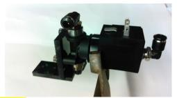
**Step 2:** To disassemble the solenoid use a Crescent Wrench to grab the metal collar next to the electromagnet body.
