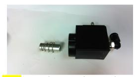
Step 4: Remove the piston and spring to clean.
