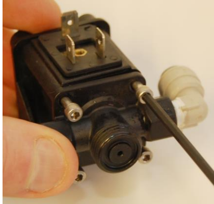
Step 2: Using a 7/64" hex wrench remove all 4 bolts that hold the spray head solenoid together.
