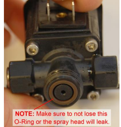
Step 3: Make sure to not lose the O-Ring (it may stick to the nozzle tip) when disassembling the unit.
