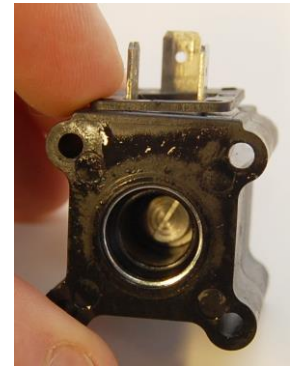
Step 3: Make sure to not lose the O-Ring (it may stick to the nozzle tip) when disassembling the unit.
