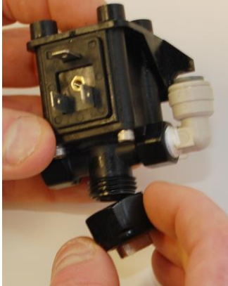
Step 1: Remove the black spray tip nut that holds the spray tip against the solenoid.
