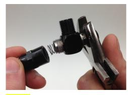
STEP 6: Next, remove the left side (Fluid Side) of the Spray Valve Assembly using the wrenches, as seen above. Remove all components and clean.
