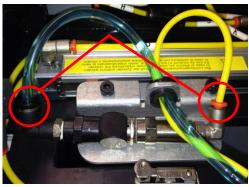
**STEP 3:** Remove the Spray Valve from the ViperONE. Do this by releasing the yellow Air line and the blue Fluid line that are connected to the Spray Valve on either end.
