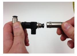
STEP 5: Remove the pneumatically activated switch from the Spray Valve.
