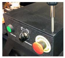
**STEP 1:** First remove all 8 screws from the top of the ViperONE. Remove the lid.
