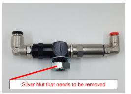
**STEP 2:** Loosening the silver nut found inside the spray chamber of the ViperONE (the bottom side of the spray head carriage as seen in STEP 3).
